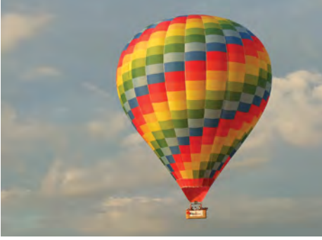
Heated air inside a hot air balloon causes the balloon to rise due to convection.
